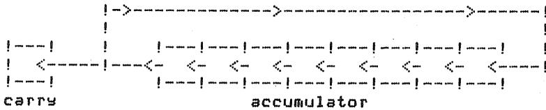
Each bit is moved one position to the left. The high-order bit goes to both the low-order bit and to the carry flag.
