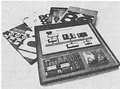
Obr. 63. Stavebnice SDK-80 firmy Intel
